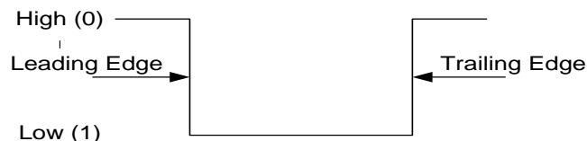
Fig. 4.4: Illustration of negative logic
