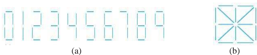
Fig. 4.134: (a) Displays the digits by an appropriate combination of lighted segments (b) The 16-segment display commonly used for alphanumeric data
