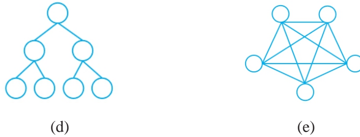
Fig. 4.141: (a) Bus topology (b) Star topology (c) Ring topology (d) Tree topology (e) mesh topology
