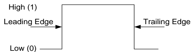
Fig. 4.3: Illustration of positive logic
