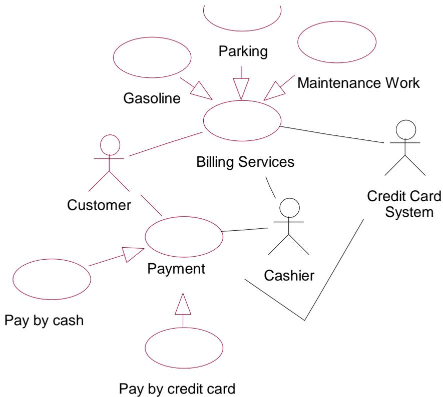
The team decides to use an Object-Oriented methodology to create the design. The figure above shows the first draft of the use case diagram for the gas station system, created during high-level (conceptual) design. Use it to answer questions 24 through 26.
