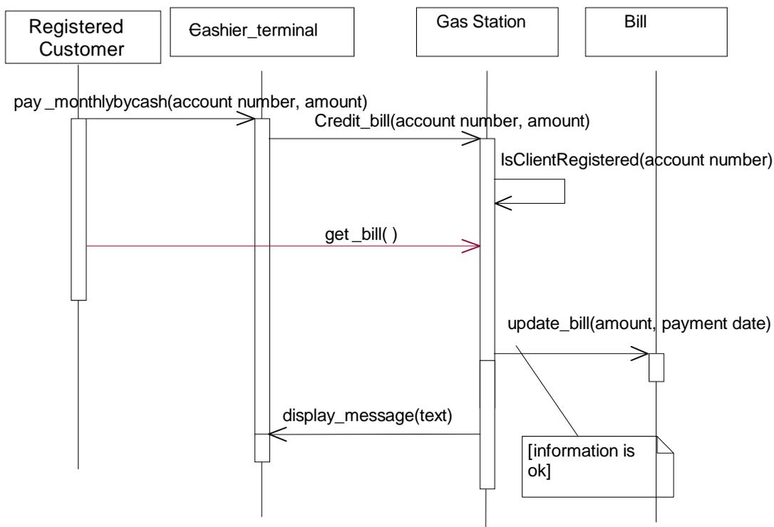
The figure above shows the first draft of a sequence diagram for the gas station system. Use it to answer questions 7 and 8.
