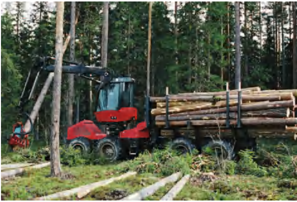
Figure 8 A Combi-machine or HarWader for combined harvesting and extraction. Reproduced with permission from Partek Forest, Sweden.
