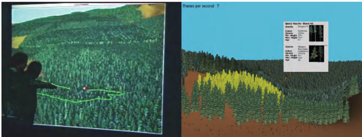
Figure 14 An interactive visualization system prototype (CALP Forester) that allows the user to prescribe management actions through a laser pointer interface and query the underlying model data. Image by Duncan Cavens, CALP.
