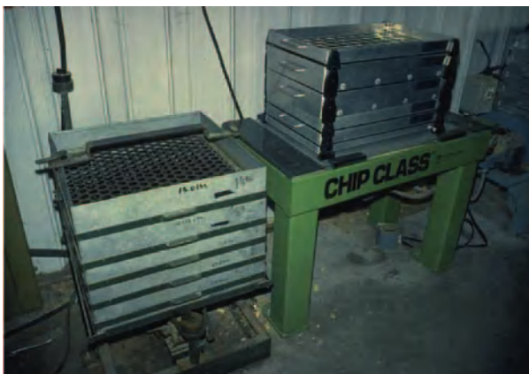
Figure 22 Chip Class classifier. The classifier next to the Chip Class is the Williams Classifier. It is the earliest classifier that the industry adopted as a standard. It is based on round holes only.
