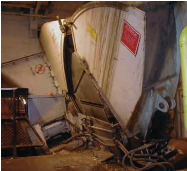
Figure 8 Woodroom chipper with hood raised for knife changing. The knife slots and knives reach from the hub to the edge of the chipper.
