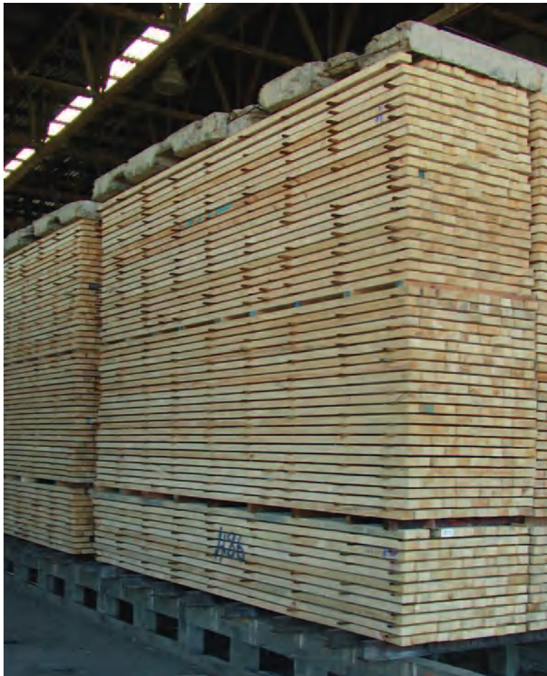
Figure 1 Lumber is stacked in cuboid packages with the layers separated by stickers so air can move between the layers.
