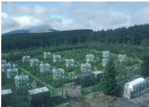
Figure 3 Open top chambers (OTCs) at Glendevon, Perthshire, Scotland. Half of the chambers are flushed with ambient air and half with ambient air with additional CO 2 added to maintain a CO 2 concentration of twice ambient. The CO 2 tank can be seen in the foreground. The control room is just inside the site gates, and a nonchamber control area containing four plots with trees but no chambers can be seen at the rear, right of the photograph. This area was included to assess the affects of the chambers themselves on the trees. Photograph courtesy of the Forest Research Photo Library.
