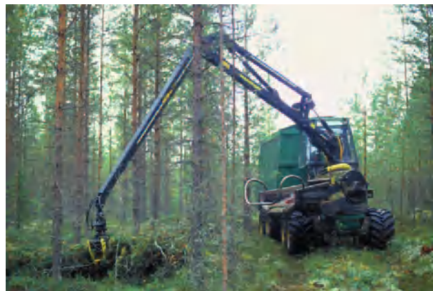
Figure 1 Moving on the corridors, a chip forwarder picks up whole-tree bunches, chips them on site, and takes the chip to a landing.
