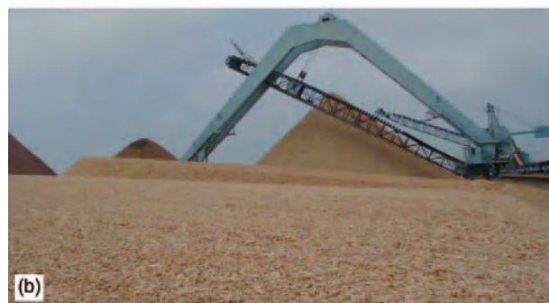
Figure 18 State-of-the-art chip storage systems. Automated outstocking and reclaim is used to maintain a first-in/first-out pile rotation. The arrangement is either circular (a) or linear (b).
