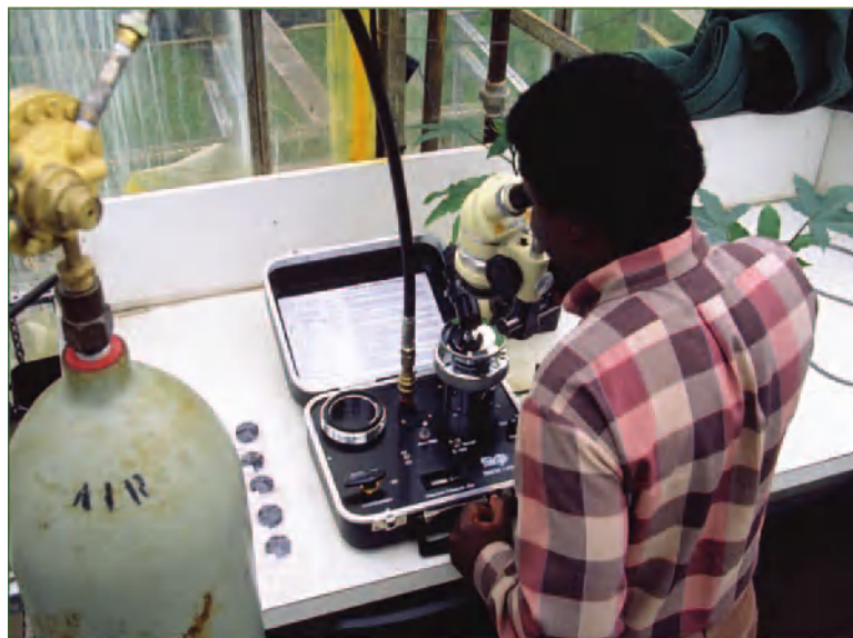
Figure 4 Using a 'pressure bomb' to assess the leaf water potential of Triplochiton scleroxylon cuttings.
