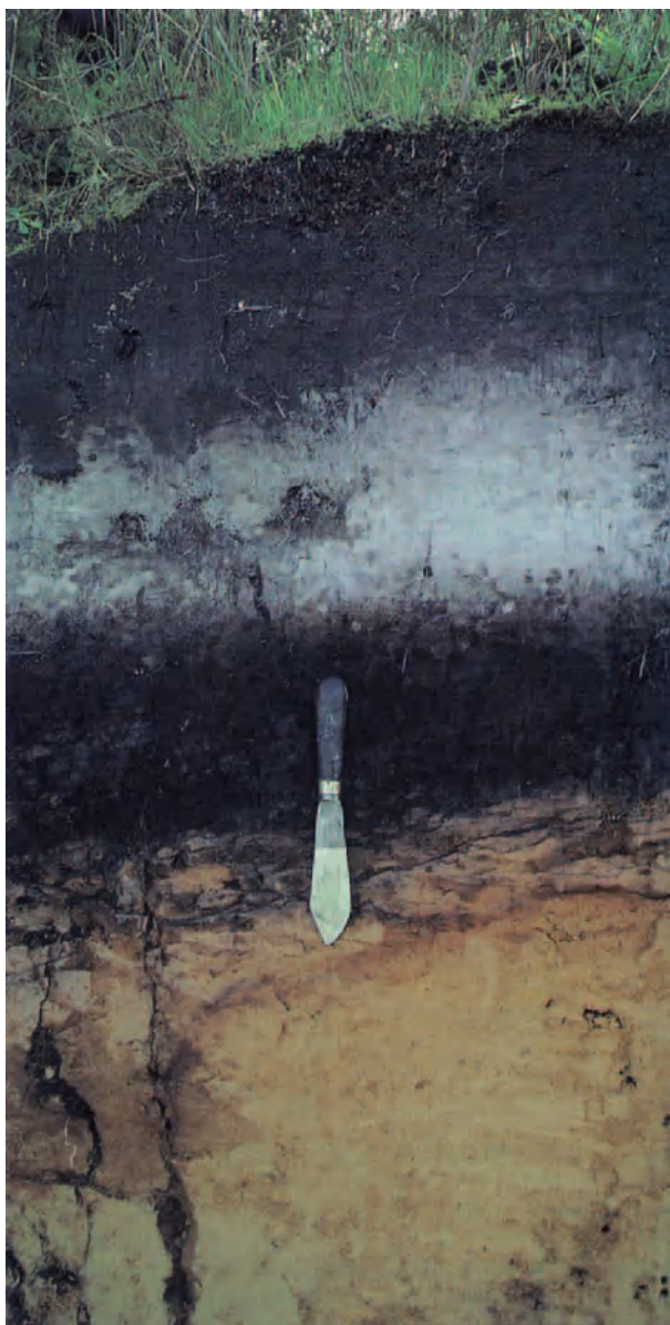
Figure 2 An 'egg-cup' podzol formed under the stems of long-lived trees in New Zealand, where extra leaching of water down the stems of Kauri trees results in distinct zones of leaching and accumulation. Reproduced with permission of the New Zealand Soil Science Society.
