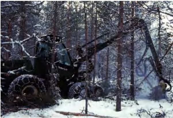
Figure 8 Standard harvesters can be used in thinning operations as well as in maturity cuts.
