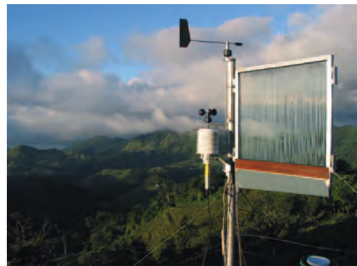
Figure 4 Wire harp to estimate occurrence of fog and wind-driven rain in northern Costa Rica. Photograph courtesy of K.F.A. Frumau.
