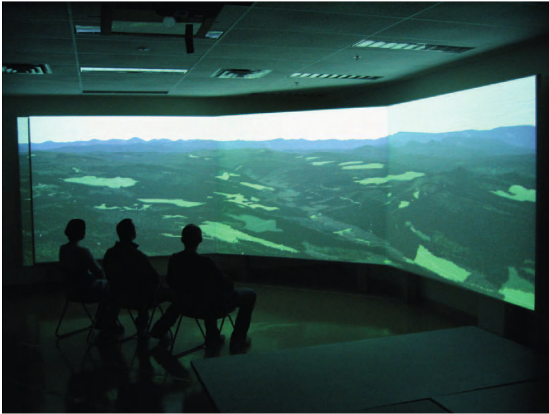
Figure 12 Immersive static image presented on three wraparound screens in the Landscape Immersion Laboratory of the Collaborative for Advanced Landscape Planning (CALP) at the University of British Columbia's Faculty of Forestry. Image by Jon Salter, CALP.
