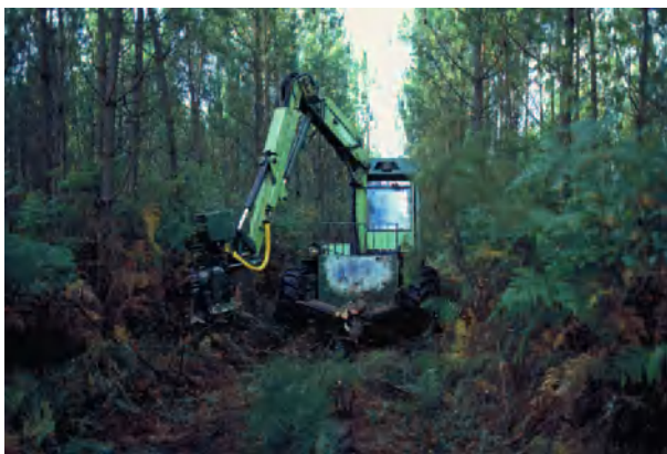
Figure 6 In early thinning, harvesters generally move along corridors, selectively thinning the stand on both sides.
