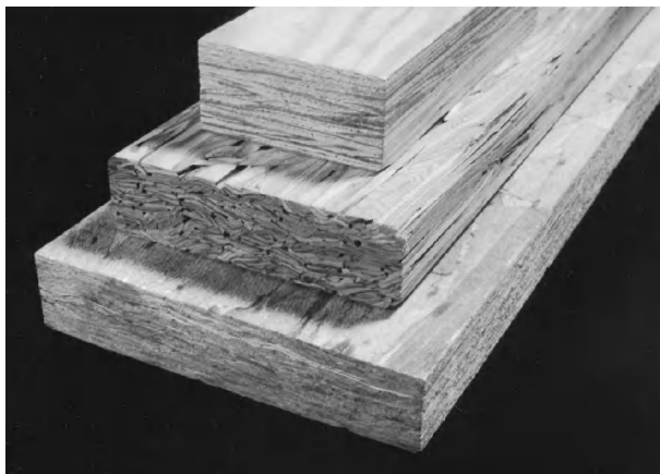
Figure 1 Examples of three types of SCL (top to bottom): laminated veneer lumber (LVL), parallel strand lumber (PSL), and oriented strand lumber (OSL).
