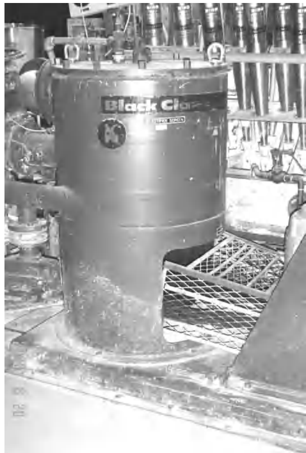
Figure 10 Pilot plant pressure screen manufactured by Black Clawson. The screen uses a slotted screen to remove contaminants from the pulp slurry.
