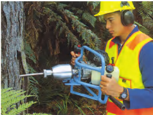
Figure 6 Sampling a Pinus radiata candidate for selection for determining several key wood properties by taking a core of 12 mm diameter. Courtesy of New Zealand Forest Research Institute Ltd.
