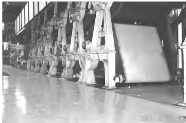
Figure 16 Dryer section of the pilot papermachine at SUNY College of Environmental Science and Forestry. The sheet passes alternately over and under steam-heated cylinders in a serpentine pattern.
