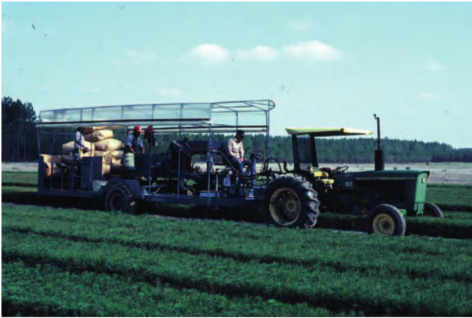
Figure 3 Mechanical lifting of slash pine ( P. elliotii Engl.) in the southeastern United States. This nursery produces 1 + 0 bareroot stock that is sown in April (spring) and is lifted 8–10 months later during winter. The machine lifts the entire seedbed in one pass. In this example, packing in bags is done in the field as opposed to transporting to a central processing area.
