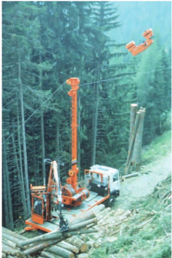
Figure 4 Steep slopes hamper timber harvesting. Cable crane logging is a suitable technology developed for mountain forests. Photo courtesy of F Frutig.
