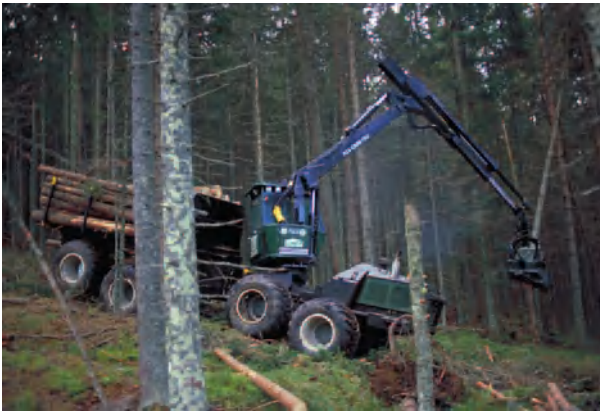
Figure 2 The integral harvester–forwarder is a new machine being introduced to thinning operations.
