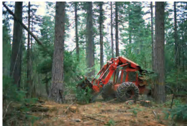
Figure 4 Compact feller–buncher in a late thinning.
