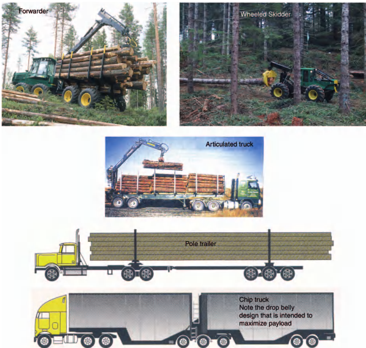
Figure 10 Categories of machines and trucks used in wood delivery. Reproduced with permission from Forestry Contractors Association, UK, and Timberjack OY, Finland.
