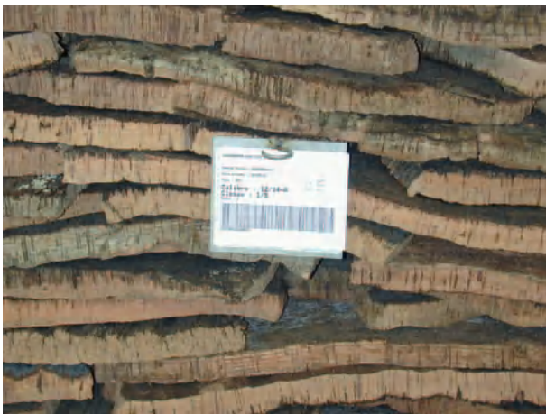
Figure 9 Cork planks after the water-boiling operation.
