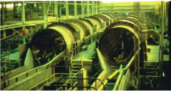
Figure 4 Long-log drum debarkers in an area with cold climate where equipment must be enclosed for winter operation.
