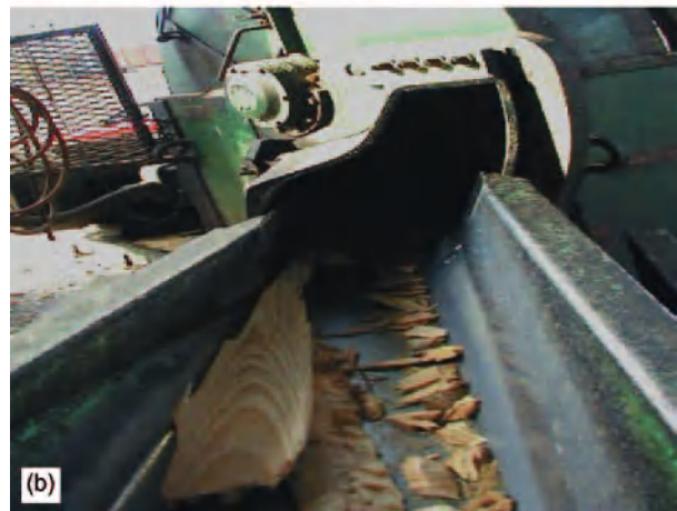
Figure 5 Sawmill chipper infeed. Vibratory conveyors are commonly used to convey sawmill waste to chippers. The size and shape of sawmill by-products varies widely. Some flows are relatively uniform (a) while others contain long slabs, trim blocks, and chip screen oversize (b). uniform sawmill chipper feed material produces more uniform chips.
