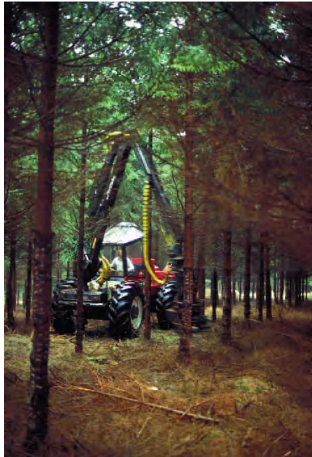
Figure 7 Dedicated thinning harvester in a row plantation.
