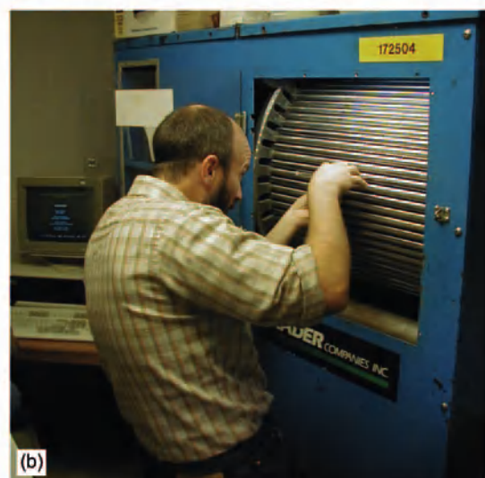
Figure 23 Rader CC2000 classifier. (a) Two systems allow much more productivity from the chip testing laboratory; (b) like all instruments, it must be periodically cleaned and carefully calibrated.
