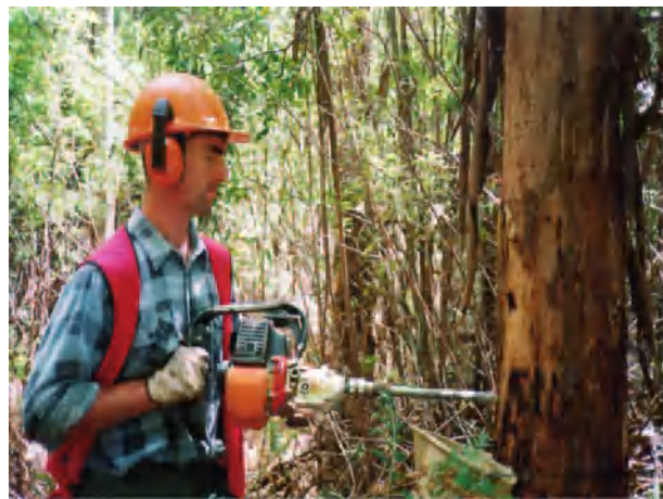
Figure 2 Coring Eucalyptus globulus for wood density assessment using a mechanized coring machine. Photograph courtesy of Carolyn Raymond, Cooperative Research Centre for Sustainable Production Forestry.
