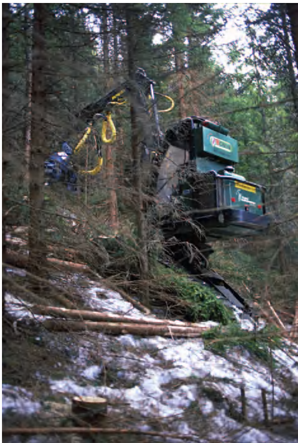
Figure 11 Self-leveling thinning harvester for steep-terrain operations.
