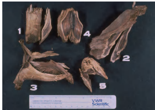
Figure 17 Oversize chips after kraft pulping. (1) Overthick chip with partial impregnation and a woody center; (2) overlength and over thick chip with only the first few millimeters on the outside that are pulped; (3) the distorted grain and compression wood near a branch created an oversize that has only surface pulping; (4) an over thick chip with a woody center; (5) knotwood creates a badly formed chip that only pulps on the surface.
