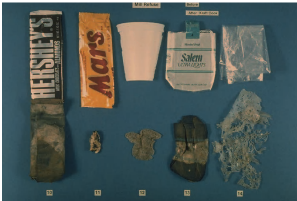
Figure 15 Common plastic items shown before and after kraft pulping. The wrapper on the far left is made of paper and will become part of the fiber furnish. The plastic bag at the far right has become a brittle lattice that will break easily in pulp handling and contaminate several hundred tons of pulp.
