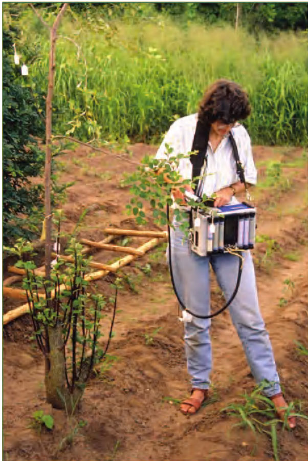
Figure 8 Using a portable gas analyzer to assess rates of pre-severance net photosynthesis and transpiration in stockplants of Zizyphus mauritiana .
