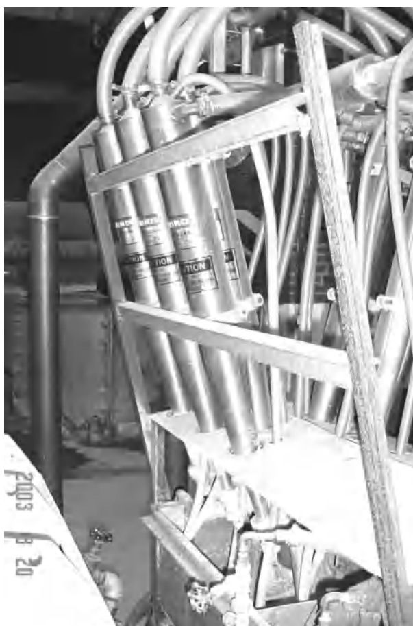
Figure 8 Pilot plant hydrocyclone cleaners manufactured by Bird. Density differences allow the removal of the heavier contaminants.
