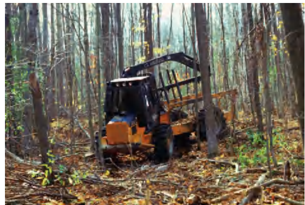
Figure 10 Specifically designed for thinning, this small forwarder can sneak into the residual stand without damaging the trees.
