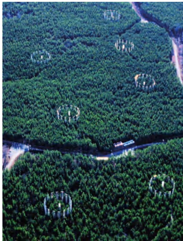
Figure 4 The free air CO 2 enrichment (FACE) rings in loblolly pine, North Carolina, USA. Three of the rings are flushed with ambient air and three with ambient air to which 200 ppm CO 2 is continually added. (The ring in the distance is a prototype.) The towers shown support white pipes with perforations for emitting CO 2 into the forest stand. Each 30 m diameter ring uses feedback control technology to control the CO 2 concentration.
