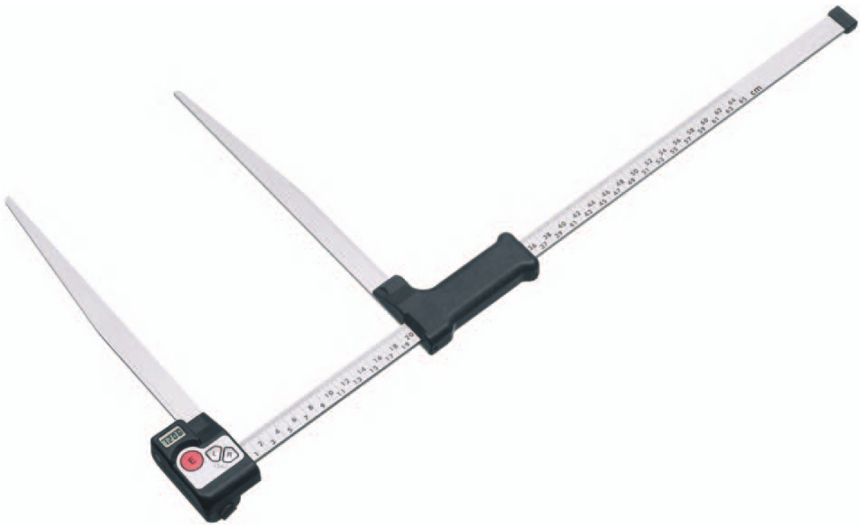
Figure 4 The caliper is the most common instrument in forest measurements. It is used for direct measurement of diameter of stems, branches, stumps, and roots. The conventional forestry caliper consists of a graduated bar with two parallel arms at right angles; one arm is fixed on the bar, while the other slides on it. Calipers made of metal or carbon fiber are more reliable than those made of wood, because they are sturdy, weather-proof, and easy to clean for resin and dirt. Modern calipers operate electronically with data storage directly in the caliper or data transfer to a portable field computer.
