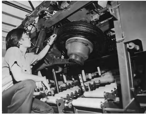
Figure 4 Manufacturing a radial-ply tire. Photograph courtesy of Tun Abdul Razak Research Centre.
