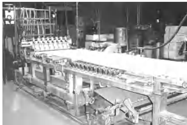
Figure 12 Wet end of the pilot papermachine at SUNY College of Environmental Science and Forestry. A hydraulic headbox is seen in the background and the forming sheet would move left to right while water drains through the wire.
